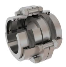
Gear coupling is composed of inner toothed sleeve and outer toothed hubs which have the same quantity of teeth, and other components. When in motion, relative displacement occurs between two shafts, and the faces of inner & outer teeth move relatively in axial direction.
