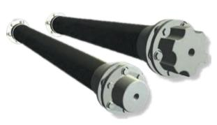
The composite material adopted is only 20% the weight of steel material, so the length of the coupling shaft of composite material is 80% longer than that of steel, and no support bearings are required. This is a kind of coupling specially designed for cooling tower fans.
